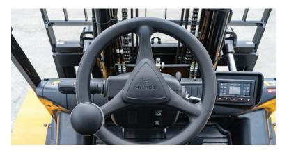
The steering wheel diameter has been reduced by 40 mm to minimise driver fatigue. A Danfoss 4th generation Orbitrol steering unit has been added to reduce noise and improve rotation.
