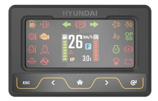
The large, clear digital display allows the driver to check operating conditions in real time. An LPG reserve lamp is included as standard and various additional functions are included for safe and convenient equipment management. These include control service interval for consumables and display of the load on the forks (OPT).
